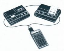
This module plugs into any of the four ports of the HP-41C/CV. Once plugged in, it allows, with simple HP-41 commands, control of up to 30 HP-IL devices.
