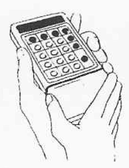
1. Grasp main body of machine firmly at indicated position and slide battery pack out.
