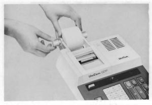
1. While lightly pulling the paper holder shaft sidewise, try to turn the shaft: this will disengage the shaft.
