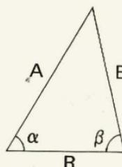
$$\frac{A}{\sin \beta} = \frac{R}{\sin (180^\circ - \alpha - \beta)} \quad \therefore A = \frac{R \times \sin \alpha}{\sin (\alpha + \beta)}$$
