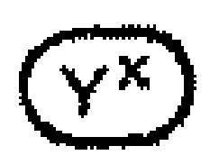
This key is used to raise to any power the numeral entered before depression of the  $y^x$  key, in the exponent of the numeral entered after depression of the  $y^x$  key.
