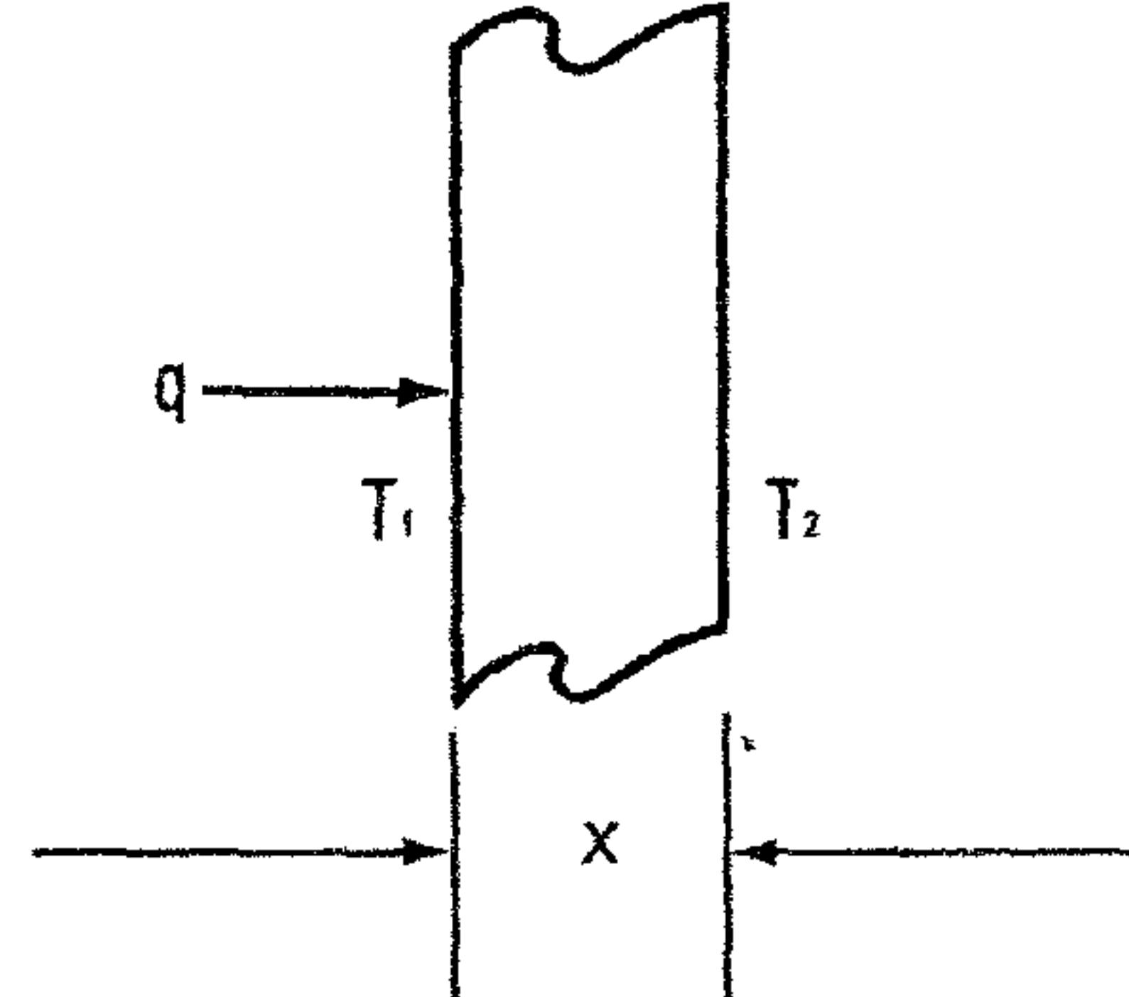
$$q = kA \frac{T_1 - T_2}{x}$$
