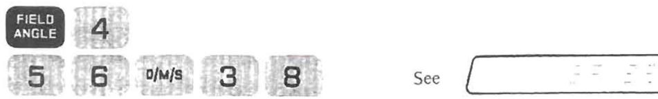
\*NOTE: The Field Angle numerical code appears in the left side of the display. The same basic key sequence holds true for the two other horizontal Field Angles.
