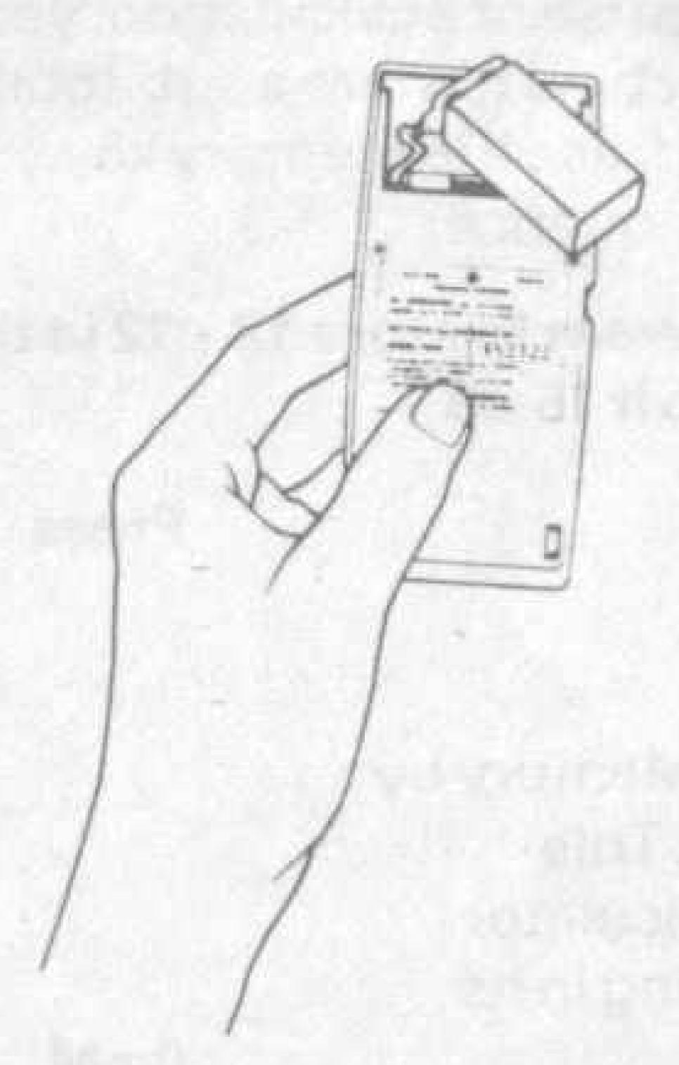
3. Unclip the leads and fit the new battery. The terminals are designed to make it impossible to fit wrongly. Press the terminal cap firmly down and check that a secure contact is made.
