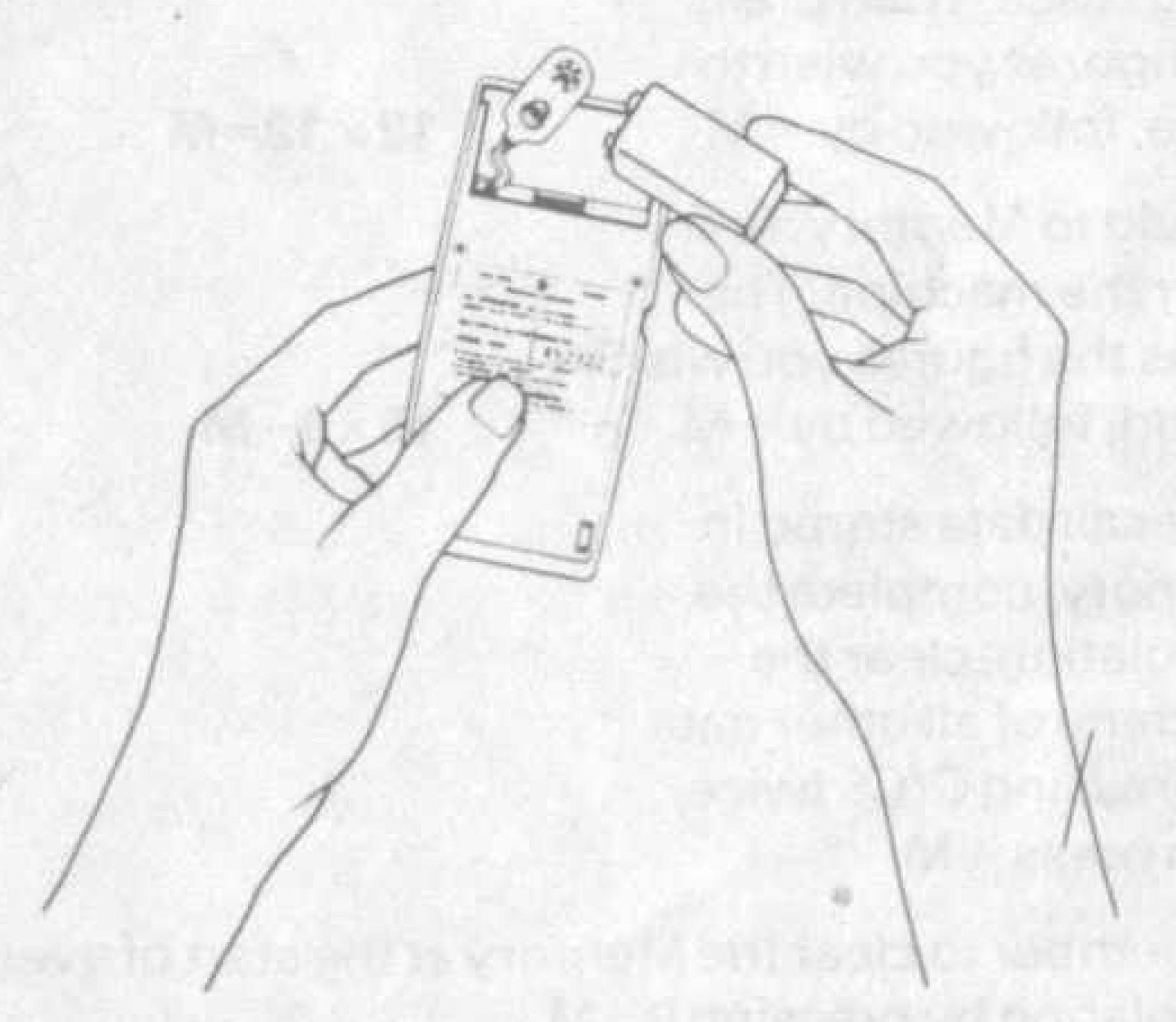
4. Fit the new battery into its compartment and slide the back panel into place.
