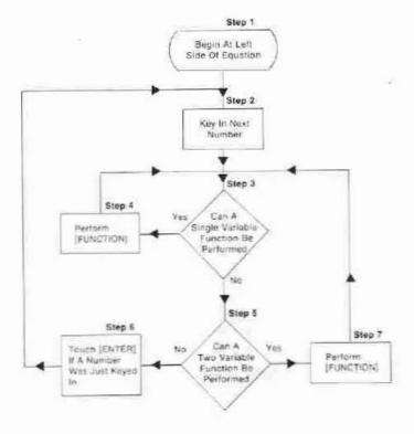
NOTE: During Step 6, you only have to touch [ENTER] if the number was just keyed in. Whenever the display contains the result of a Function, it is not necessary to touch [ENTER] before keying in a number.
