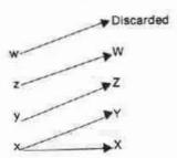
Single Variable Functions - Functions such as x² are called single variable functions since they only require a single operand in order to be performed. When a single variable function is performed [F(x)], only the contents of the X register are effected.
