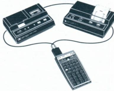
This module plugs into any of the four ports of the HP-41C/CV. Once plugged in, it allows, with simple HP-41 commands, control of up to 30 HP-IL devices.
