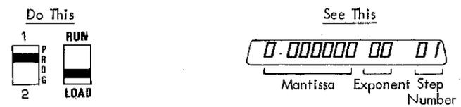
The number at the far right of the display tells you which step of the 80-step memory is ready for loading. On the left side of the display is the mantissa and between the mantissa and the step number is the two digit exponent to the mantissa. When in LOAD, all numbers are displayed in scientific notation. Your main concern is with the step numbers. The mantissa could be anything depending on what you have done prior to loading your program.
