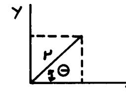
The legends on the keys tell you how to do it. Enter  $x$ , poke the To Polar key, enter  $y$  and poke  $=$ . The first value ( $\theta$ ) will be on the display, 2ND FUNC will give you  $r$ .
