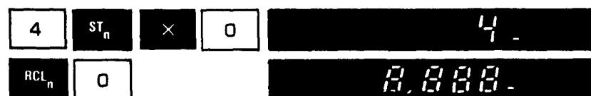
Easy? Just remember to push **ST<sub>n</sub>** before the arithmetic key, the register number after.
