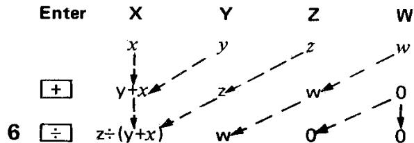
The **entry key ENT** is used to enter numbers into the operational chain. Each time you press ENT you rotate the chain as shown below. The ENT key should be immediately followed by a numerical entry (see note on page 11).
