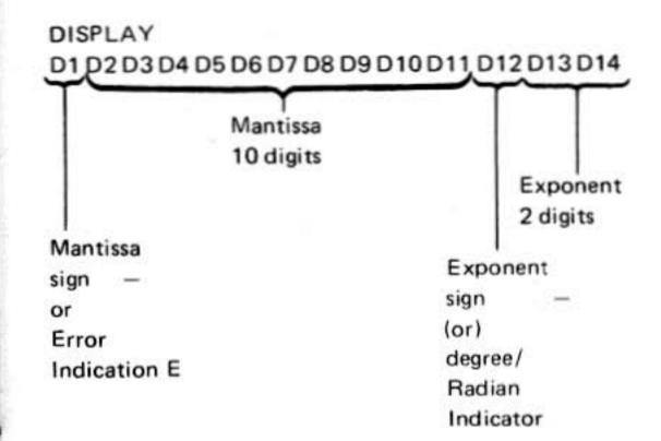
The decimal point of the last exponent digit indicates the angular unit mode selected by the d/r and  $F \xrightarrow{d \leftrightarrow r}$  keys: degrees when off or radians when lit.
